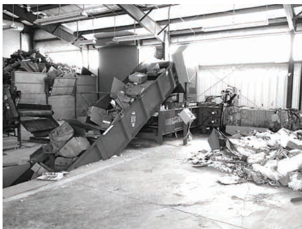
SSWA BALER AT WORK COMPRESSING CARDBOARD FOR RECYCLING AT THE LANDFILL SOUTHWEST OF SILVER CITY. (JEFF WHITKAMP PHOTO)
